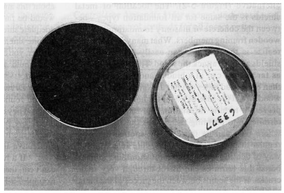
Figure 5-1. Short term radon canister.
